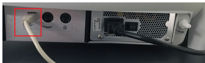
Figure 1: Connect supplied USB cable to the back panel of the Evolution.
