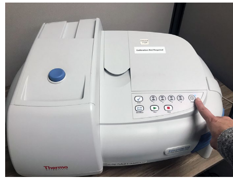
Figure 6: Remove the dosimeter holder from the baseplate. Close lid of Evolution before powering on the instrument.
