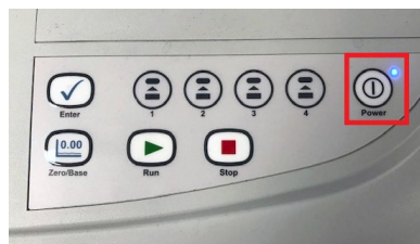
Figure 4: Power on/off button on front panel of Evolution 220. Solid blue indicator light means the Evolution has completed initialization and ready for use.
