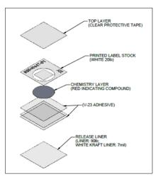
A calibrated activation chemistry layer is applied at each temperature event location on the label. The chemicals in the indicators are calibrated to react at the labeled temperatures. The label chemistry has been proven to be reliable under high-radiation dose conditions in designed experiments.
