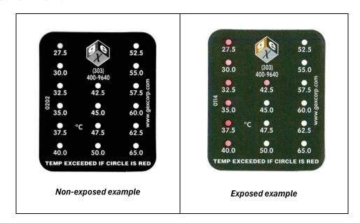
The GEX P8003 Irreversible Temperature Indicators are a self-adhering, self-activating, monitoring tool that provides a visual and irreversible record of the maximum temperature exposure. The product has a successful 20-year history of use in the radiation processing industry and is accurate flexible, non-toxic, and non-breakable Indicator of maximum temperature.
