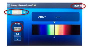
7.3.4.9 After the instrument is zeroed, insert a dosimeter to be measured, and type the absorbance value into the form for dosimeter #1.
