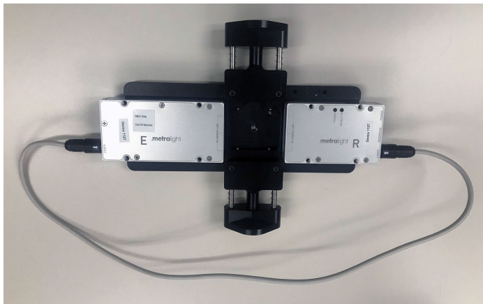
Figure 2: Emitter and Receiver connected with the Interconnect cable
