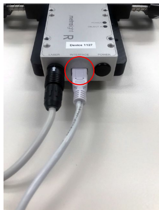
Figure 3: USB mini-interface cable attached to the “R” Receiver end of the laser micrometer
