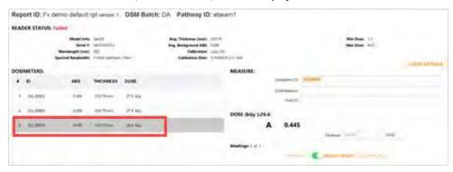
(i) Any entry done in Manual Mode is flagged as 'manual' in the database to distinguish it from automatic measurements.
