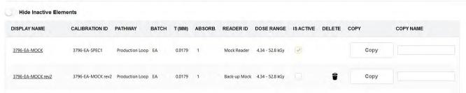
Primary reader's calibration is active; back-up reader's calibration is setup in "Calibrations"
