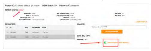
2 Type the dosimeter ID into the Dosimeter ID field on the measurement screen. Click "Add Dosimeter" button. You will see the dosimeter's ID added to the Dosimeters list without an absorbance value, thickness or calculated dose:
