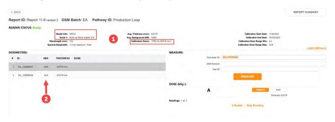
**8 Measure the dosimeters and complete the report.** The absorbance and dose for each dosimeter appears on the measurement screen, the Report Summary screen and all report outputs. Notice the reread symbol next to the dose - the software treats the measurement as a reread because any original measurement (in Report v1) is not overwritten.
