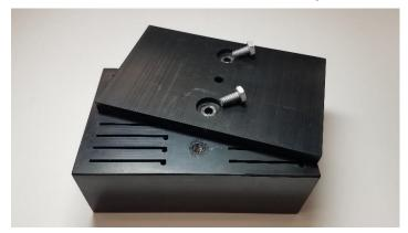
5. Attach the new shorter block to the baseplate and secure using the two bolts.
