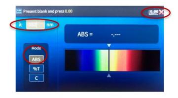
7.3.3.9 After the instrument is zeroed, insert a dosimeter to be measured, and type the absorbance value into the form for dosimeter #1.
