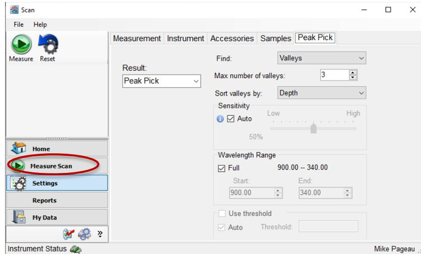
**Step 6:** Open the sample compartment lid. Ensure the Windose receiver is installed in the baseplate. Remove the dosimeter holder or any samples. Push the “Baseline” button to take a zero-absorbance scan of the empty sample compartment over the range of wavelengths.
