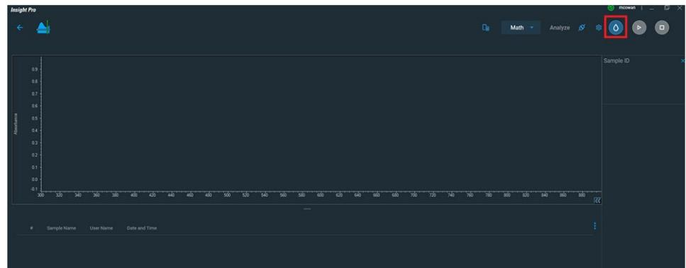
**Step 6:** The “Load Blank” prompt appears. Click “Ready” after confirming the Windose dosimeter receiver is empty and the lid is closed. The Evolution will zero.
