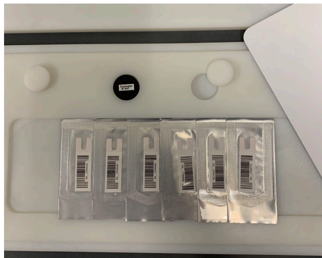
FIGURE 2: B3 dosimeters overlapping edges (with alanine dosimeter)
