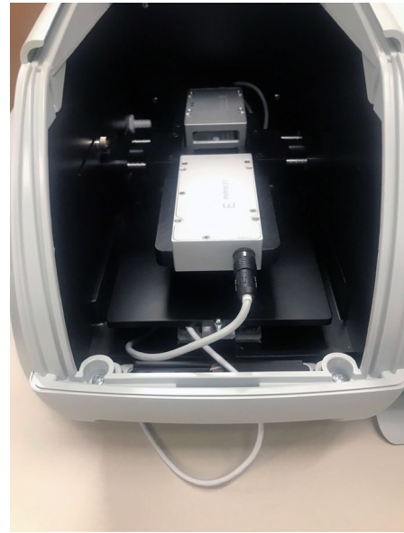
Figure 5: The USB cable threaded through the foam piece in the front of the sample compartment. The cable can now be plugged into the PC USB port
