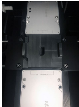
Figure 6: PMMA holder inserted into the baseplate
