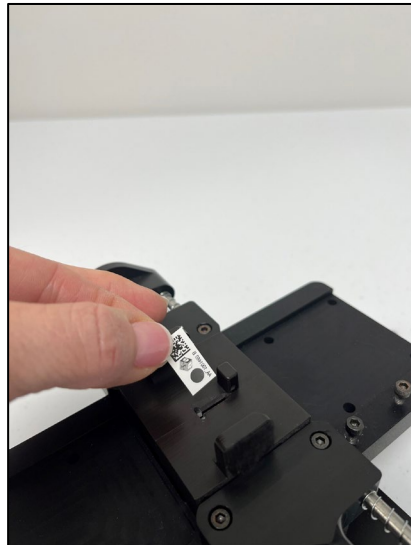
FIGURES 7 & 8 GEX B3 dosimeter placement in the P4345 dosimeter holder
