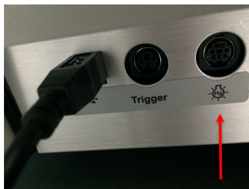
Figure 3: Mercury Lamp port on the back panel of the Evolution.
