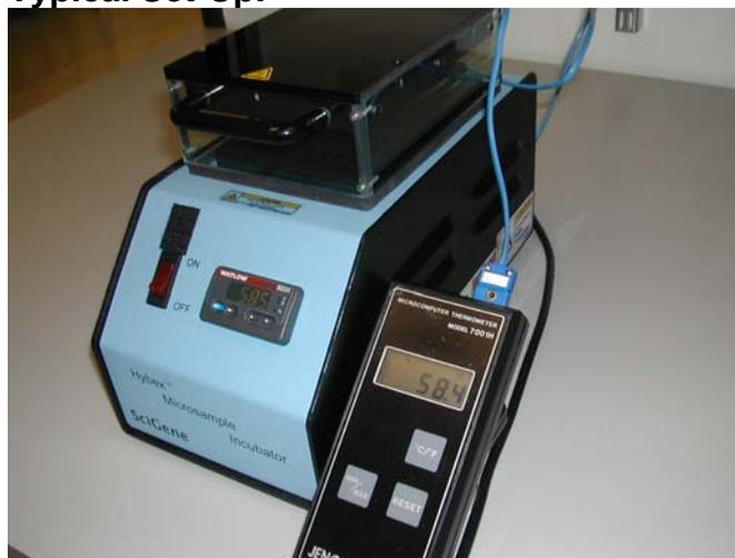
Digital Thermometer connected to Micro Incubator.
