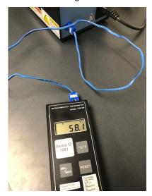
3) Turn on the thermometer. Allow 1 minute for the thermometer to stabilize. The actual temperature of the block will be displayed.
