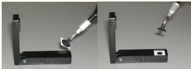
**Examine the anti-static suction tip for particulate before use. Clean with an alcohol wipe as necessary.**
