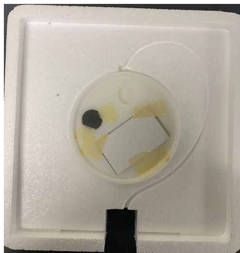
Figure 5 – Alanine Loaded & Secured
